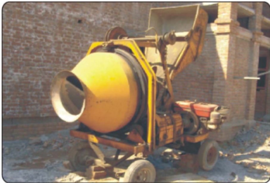
Fig. 9 Concrete aggregates mixing machine
