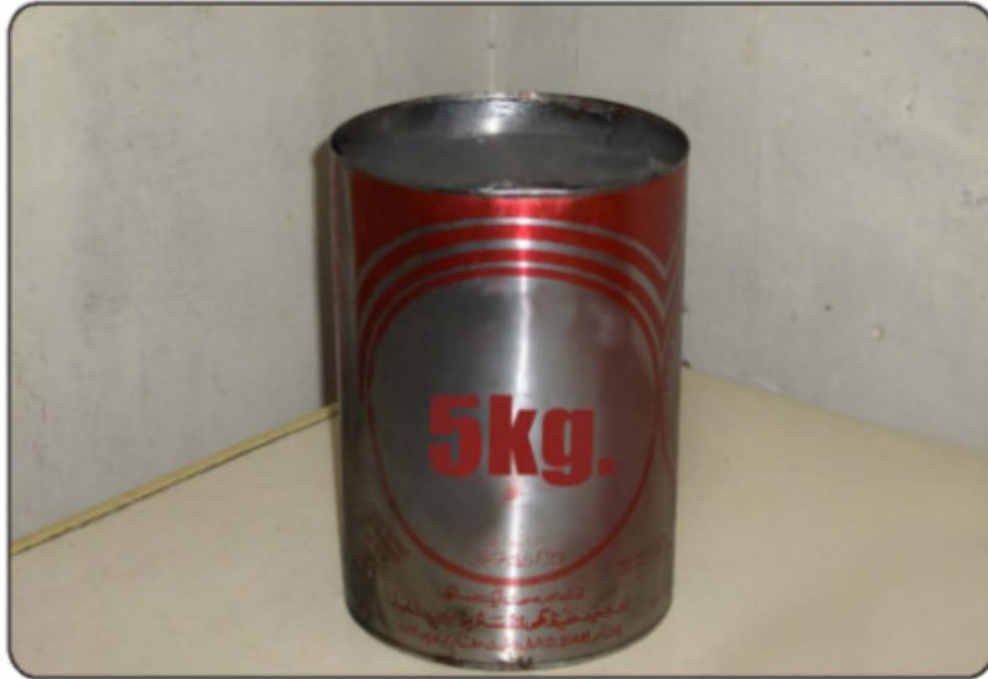
Fig.7 Five Kg oil tin to measure water for mortar and concrete
