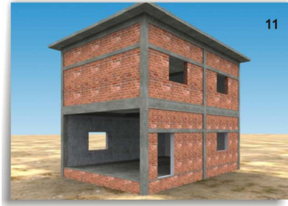
11. Complete wall masonry. Fix steel wire mesh on inner side of wall and plaster.
