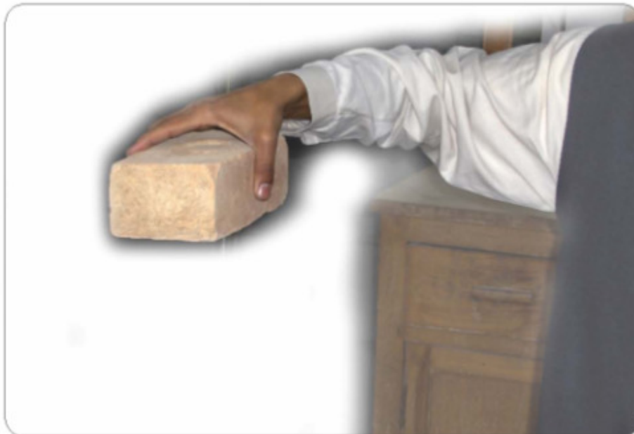
Fig.5 Dropping of brick from 4 feet height
