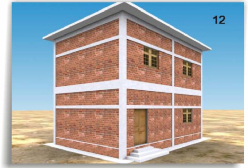
12. Fill concrete around the building to protect it from rain water.
