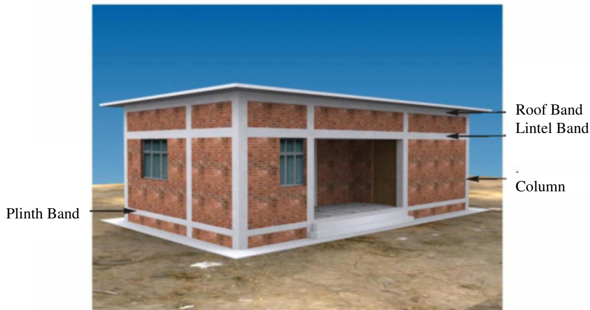
Fig.17 Columns at the corners of rooms of Building
