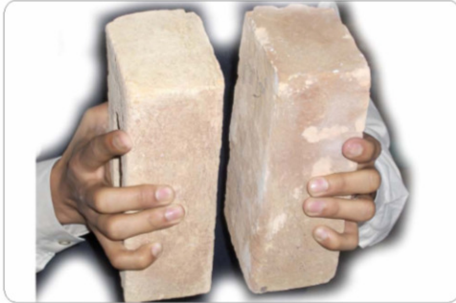
Fig.4 Striking of two bricks with each other
