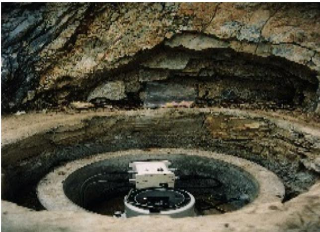
**Figure 2.** (ZM 500) Seismometer in the Vault
