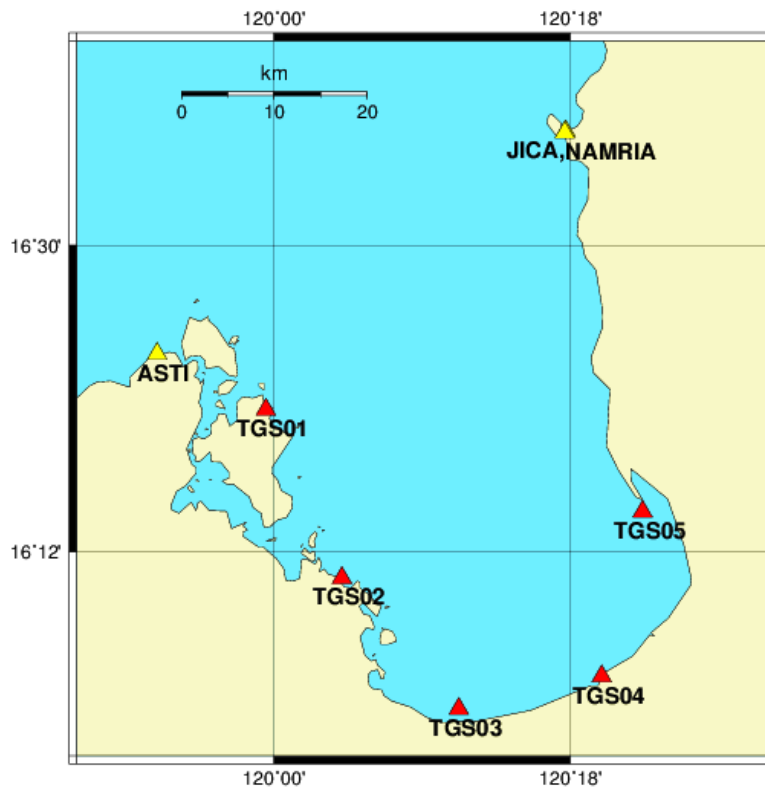
Figure 2. Location of the tide gauge stations set as output points. The yellow triangles are existing, pre-existing and proposed tide gauge stations. JICA and NAMRIA tide gauge stations are close to each other. The red triangles are assumed tide gauge stations.
