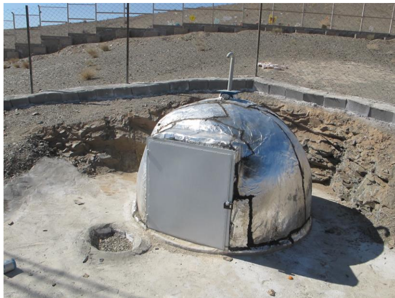
Figure 4. New dome of IRSC's station that is designed to reduce environmental noise and temperature effect.
