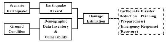
Figure 1. General flow of earthquake damage estimation
