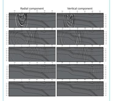
Snapshots of seismic wave fields calculated by the finite difference method from Mexican Pacific to Mexican basin (left: the radial components; right: the vertical components). Snapshots at 10, 30, 50, 80, and 100 seconds after the origin time are shown from the top to the bottom panels, respectively (Galaviz, 2017).
