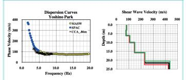
The left panel: Rayleigh-wave phase velocities derived from microtremor using the spatial autocorrelation method (SPAC: blue circles) and the centerless circular array method (CCA: crosses), and the multichannel analysis of surface waves (MASW: yellow circles). The right panel: Estimated S-wave velocity structure models by heuristic search (Black, 2011).
