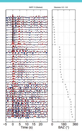
Stacked receiver functions for a broadband station (SMPP) in the Philippines for the radial component with corresponding back azimuths (Rivera, 2016).
