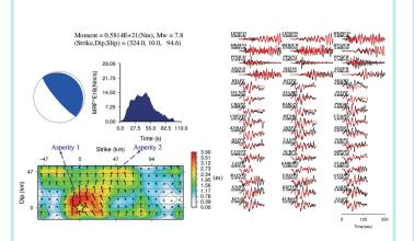
Source rupture process model of the October 25, 2010 Mentawai earthquake determined by joint inversion of teleseismic body wave and near-source strong motion data (Fatchurochman, 2011).
