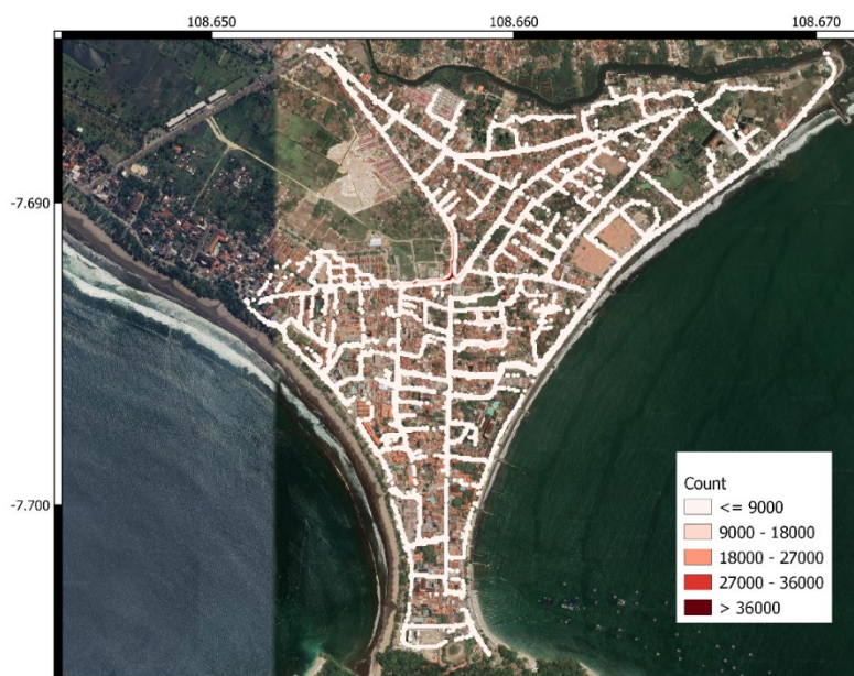
Fig 2. Congestion severity map indicates how severe the congestion is on a specific road. The higher the number (dark red), the more severe the congestion was.
