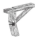
Figure 6.2: Rupture of columns at the connection of knee brace and column
