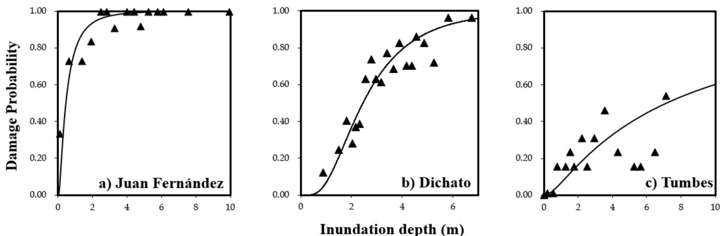
Fragility functions for structural damage in terms of the tsunami inundation depth at (a) Juan Fernandez, (b) Dichato, and (c) Tumbes.
