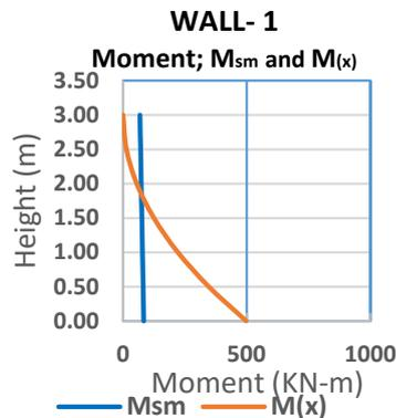
Figure.3. The overturning moment ( $M_x$ ) due to seismic action and the traditional house's Moment capacity ( $M_{sm}$ ) in out-of-plane direction. The  $M_x$  surpasses  $M_{sm}$  vastly. We should reinforce the walls to prevent overturning in this direction.
