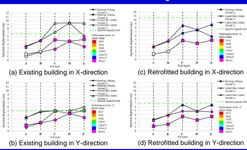
Figures (a) and (b) show the maximum inelastic displacement of the existing building in X and Y directions respectively, meanwhile figures (c) and (d) show the maximum inelastic displacement of the retrofitted building in Υ directions Х and respectively, based on the seismic hazard level at Bentong, Pahang and Lahad Datu, Sabah with profile different soil models.
