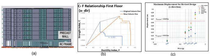
Fig. (a). Illustrates the target building's hybrid structure, featuring precast walls on its upper levels and a reinforced concrete frame on its ground floor.
