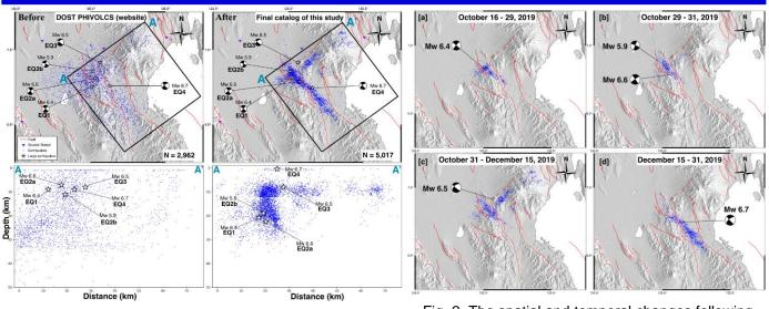
Fig. 1. Distribution of hypocenters. Routine catalog by DOST-PHIVOLCS (website) versus the final catalog of this study after applying HypoDD.
