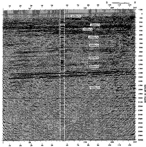
Cross section from seismic reflection survey at Shimohsa seismic observation point.
