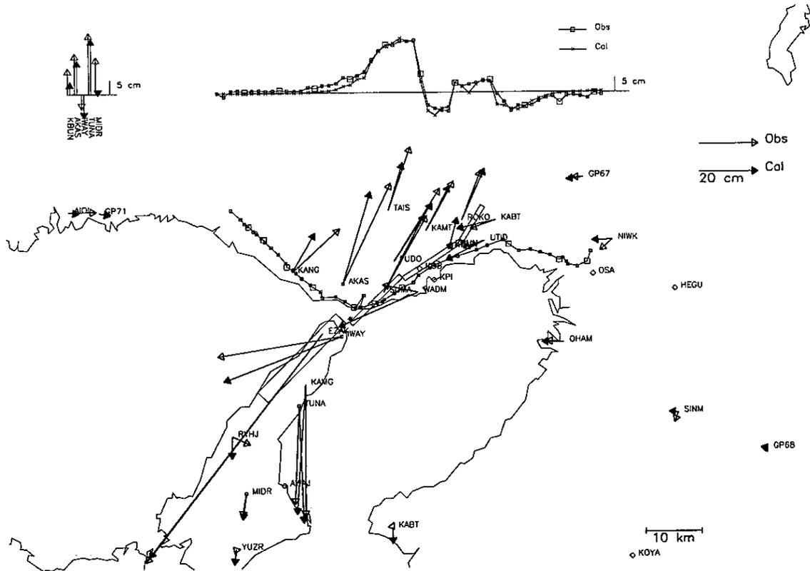
Fig. 6. Comparison between the geodetic data and calculated displacements from the inferred model (shown in Fig. 7) assuming the Nojima, Suma, Suwayama, and Gosukebashi faults.
