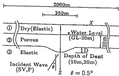
Fig.4 Configuration of studied soil medium.
