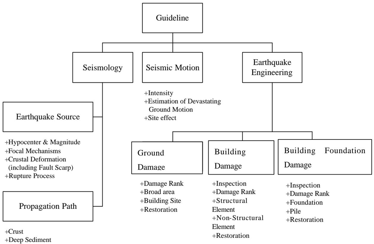
Fig. 2.1-3 Outline of Guideline for Damage Survey Methods
