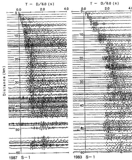
Fig. 5. Comparison of record sections for Kushigata-Shimizu Profile of 1983 and Hayakawa-Shizuoka Profile of 1987. These two profiles run parallel to each other and their spacing is only about 10 km.
