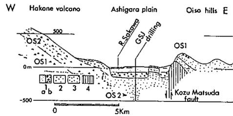
Fig. 3 Schematic Profile of the relationship between Ashigara Valley and Oiso Hills, Hakone Volcano (after Yamazaki et al., 1982)
