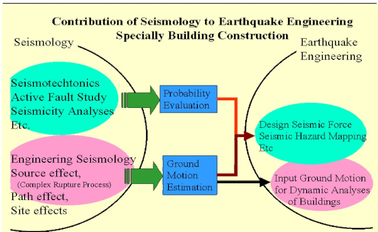
Fig. 2.1-1 Contribution of Seismology to the construction engineering
