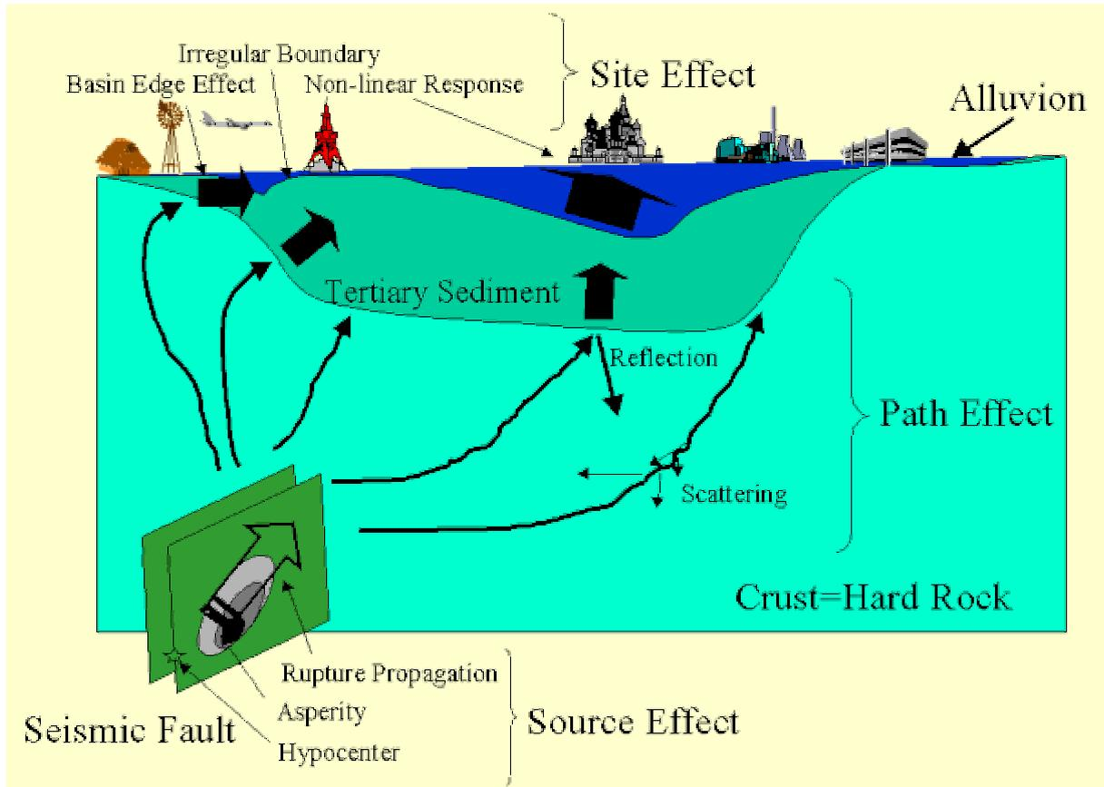
Fig. 2.1-2 Three effect composing ground motion at the surface
