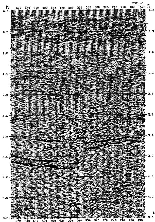
The sonic prospecting cross section at the Tokyo-Bay. The North Tokyo-Bay fault is crossing in the bedrock at the center of the figure.
