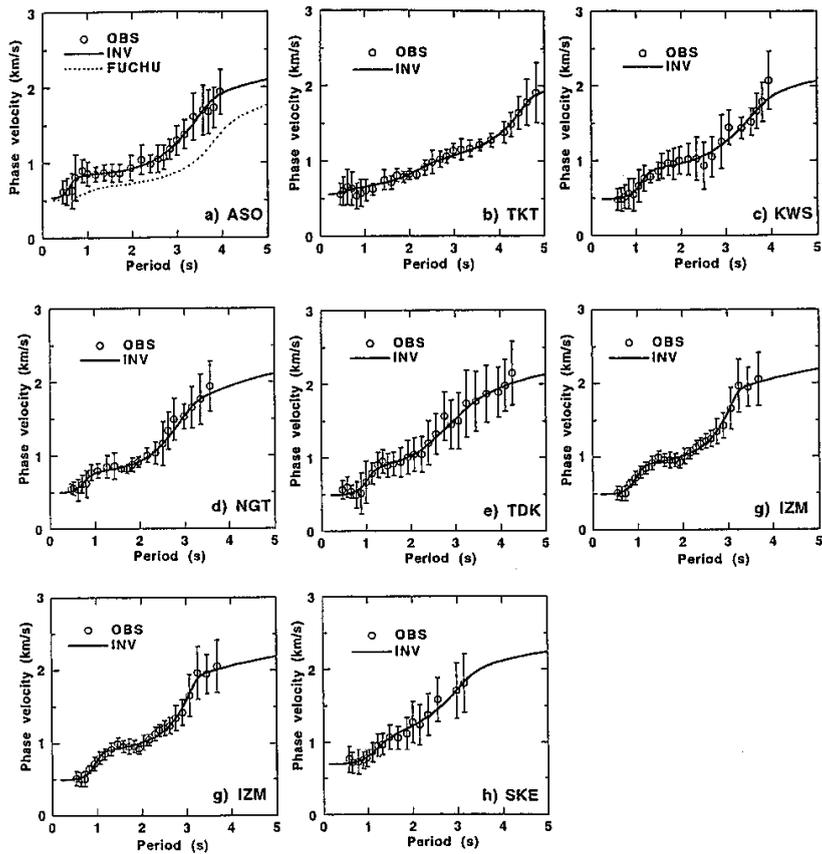
Fig. 7. Comparison of observed phase velocities with theoretical ones at all sites. Open circles indicate the observed phase velocities of microtremors with standard deviations shown by bars. Solid lines show theoretical phase velocities for fundamental Rayleigh waves in inverted subsurface structural models shown in Fig. 6.
