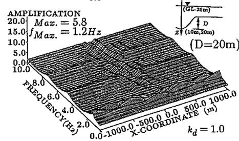
Fig.5 Frequency response characteristics on a surface due to incident plane SV wave in a layered medium with subsurface irregularity
