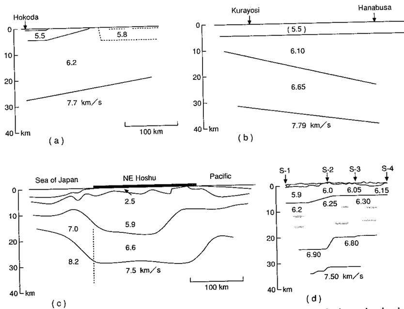
Fig. 4. Examples of crustal models in the Japanese Islands obtained from explosion seismic observations. (a) Hokoda Profile, NE Honshu [MATUZAWA *et al.* (1959)], (b) Kurayosi-Hanabusa Profile, SW Honshu [YOSHII *et al.* (1974)], (c) Kesenuma-Oga Profile, NE Honshu [YOSHII and ASANO (1972)], (d) Kuji-Ishinomaki Profile, NE Honshu [IWASAKI *et al.* (1993)]
