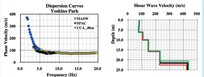
The left panel: Rayleigh-wave phase velocities derived from microtremor using the spatial autocorrelation method (SPAC: blue circles) and the centerless circular array method (CCA: crosses), and the multichannel analysis of surface waves (MASW: yellow circles). The right panel: Estimated S-wave velocity structure models by heuristic search (Black, 2011).
