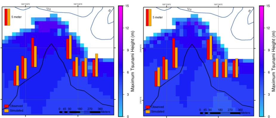
Fig 2. Comparisons between the observed tsunami heights (red bars) by Satake et al. (2012) and the simulated ones (orange bars) from the NFM result (left) generated 54 minutes after the earthquake and the forecasted model using the NearTIF method (right) obtained within 11 minutes after the earthquake. Both have similar inundation extent and tsunami height distribution.
