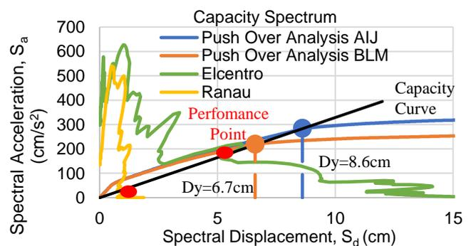
Fig. 2. Comparison of the capacity spectra of the AIJ and BLM models (earthquake).
