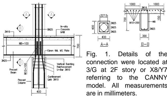
Fig. 1. Details of the connection were located at 3/G at 2F story or X8/Y7 referring to the CANNY model. All measurements are in millimeters.
