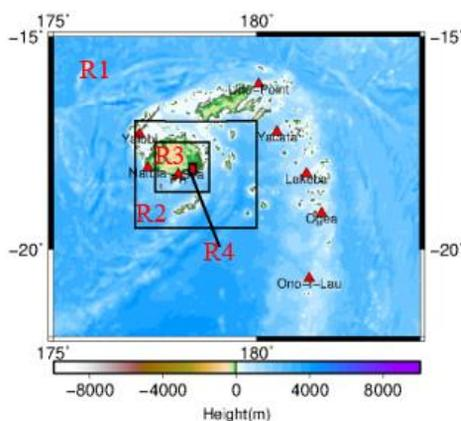
Figure 2. Nesting grids with four layers (R1 – R4) for the Suva study area.
