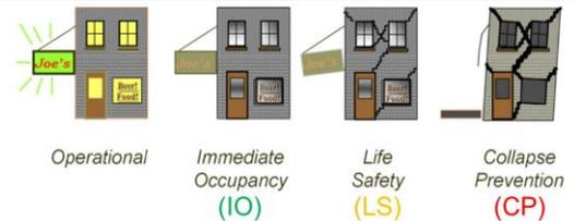
Fig. 2. Performance levels criteria (ASCE 41-17)
