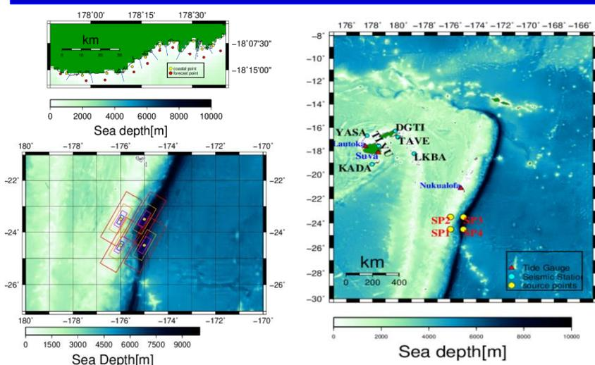
Figure 1. (top left) Distribution of Coastal Points (CPs) and Forecast Points (FPs). The blue lines divide the coastal block G around Suva into smaller regions for FP (red circles) and CP (yellow circles) pairs. (bottom left) Fault models for each Source Point (SP). The red, orange, purple and blue rectangles denote M8.5, M8.0, M7.5 and M7.0 fault models, respectively. (right) Locations of SPs, tide gauges (red triangles) and broadband seismic stations (cyan circles).
