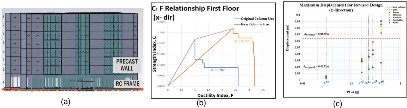
Fig. (a). Illustrates the target building's hybrid structure, featuring precast walls on its upper levels and a reinforced concrete frame on its ground floor.
