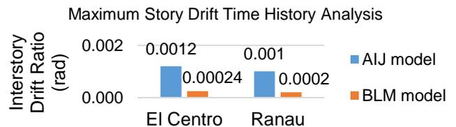
Fig. 4. Comparison of the maximum story drifts for the AIJ and BLM models with the THA
