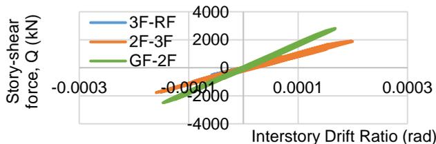
Fig. 3. Load-deformation curve for the BLM model under the Ranau ground motion. From THA.
