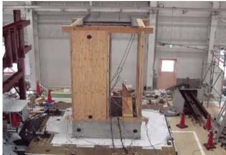
With Oil Dampers Max. Displacement= 282mm
