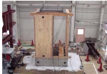
Without Oil Dampers Max. Displacement= 291mm
