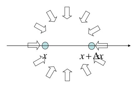
Isotropic wave field: waves come from all directions with uniform power.
