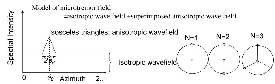
Plane wave coming from one azimuth for the discrepancy of  $\rho(r,\omega) < 0.05$  times of true value rk<3.5, i. e.,  $\lambda/r>1.8$  (N=3), rk<0.5, i. e.,  $\lambda/r>14$  (N=1 and 2)
