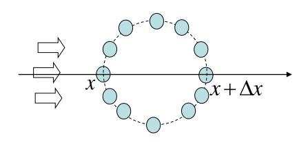
Anisotropic wave field: isotropic sensor arrangement of array observation can perform averaging.
