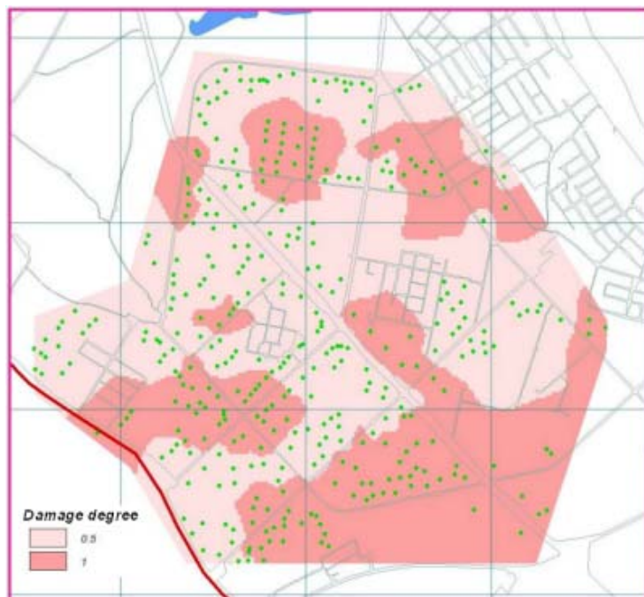
Fig.1.28. Map of buildings damages with the removed resonance effect (Kishinev, Botanica, 30.08.86).
