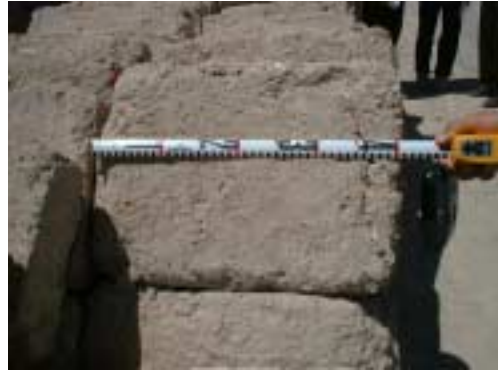
Picture 2-2-7-2. The size of adobe blocks used. The adobe walls are thinner than those used in the Centro District.
