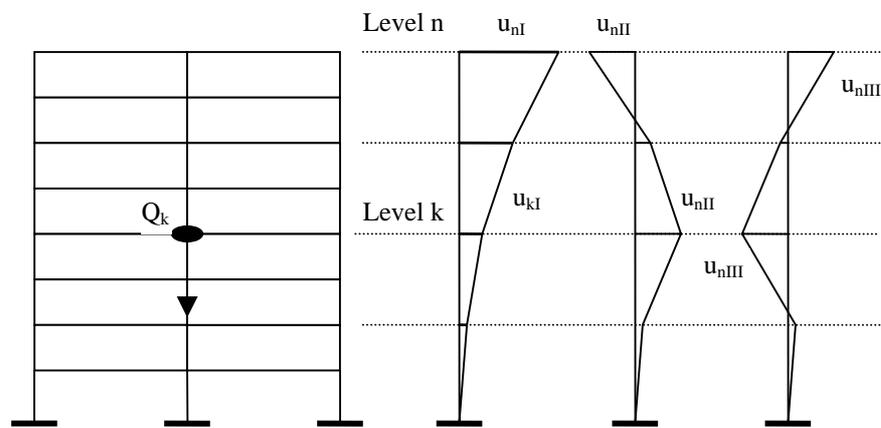
**Figure 4:** First three vibration modes
