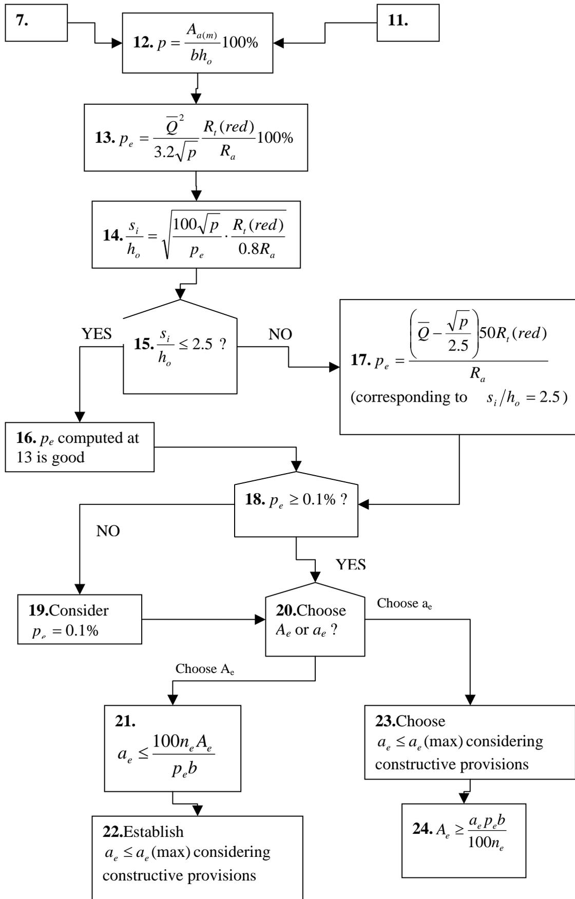
**Figure 26:** Computation of the stirrups for an element without axial force: We know  $b, h, R_t, R_a, Q, A_a$  and we are interested in  $A_e, a_e$ .
