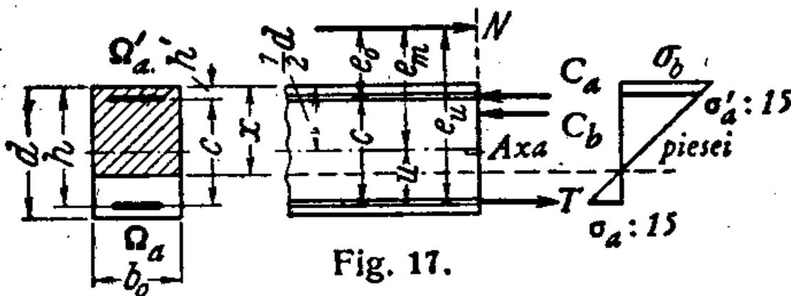
Figure 17: Double reinforced rectangular section
