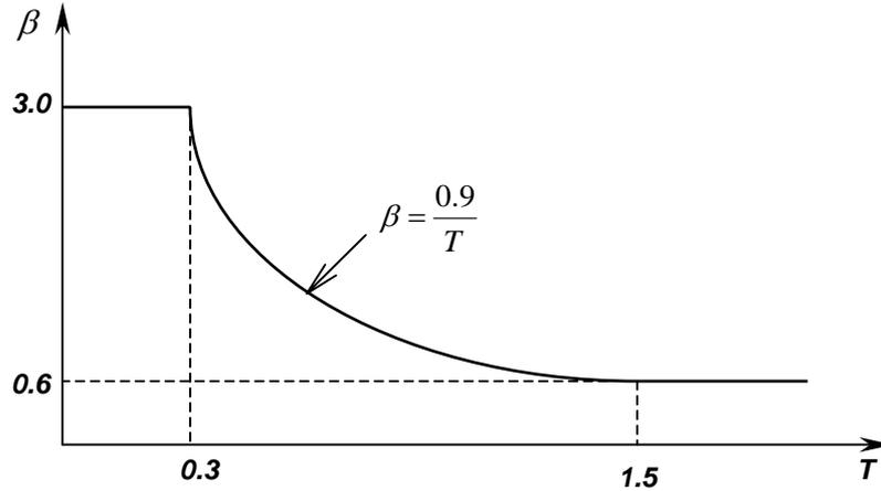
**Figure 1:** Amplification spectra
