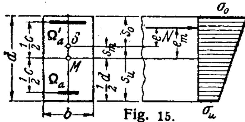
Figure 15: Concrete section subjected bending and axial force with small eccentricity
