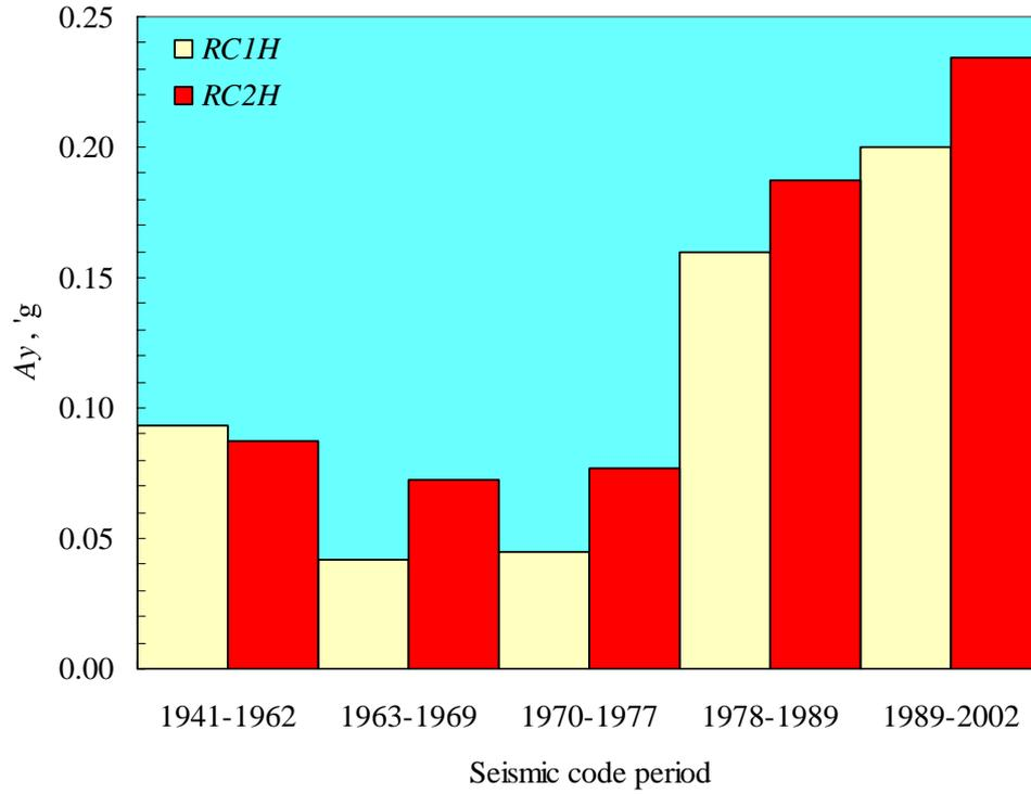
**Figure 11:** Yielding acceleration according to seismic code period
