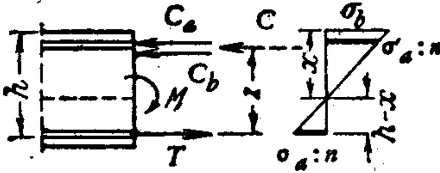
Figure 13: Simple reinforced concrete section
