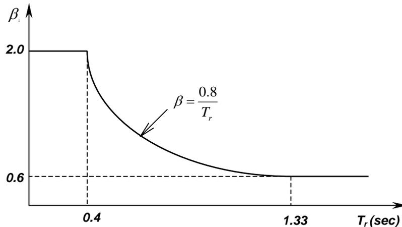
**Figure 3:** Amplification spectra
