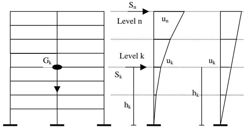
**Figure 6:** Linear approximation of the fundamental vibration mode
