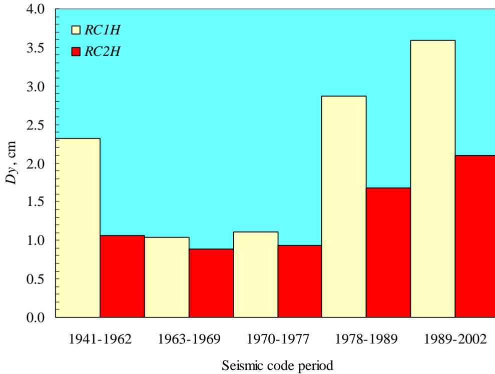
**Figure 9:** Yielding displacement according to seismic code period
