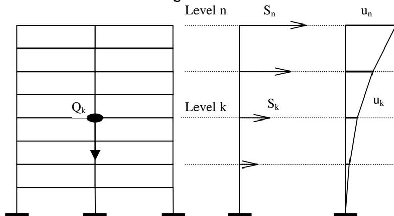
**Figure 2:** Distribution of seismic force
