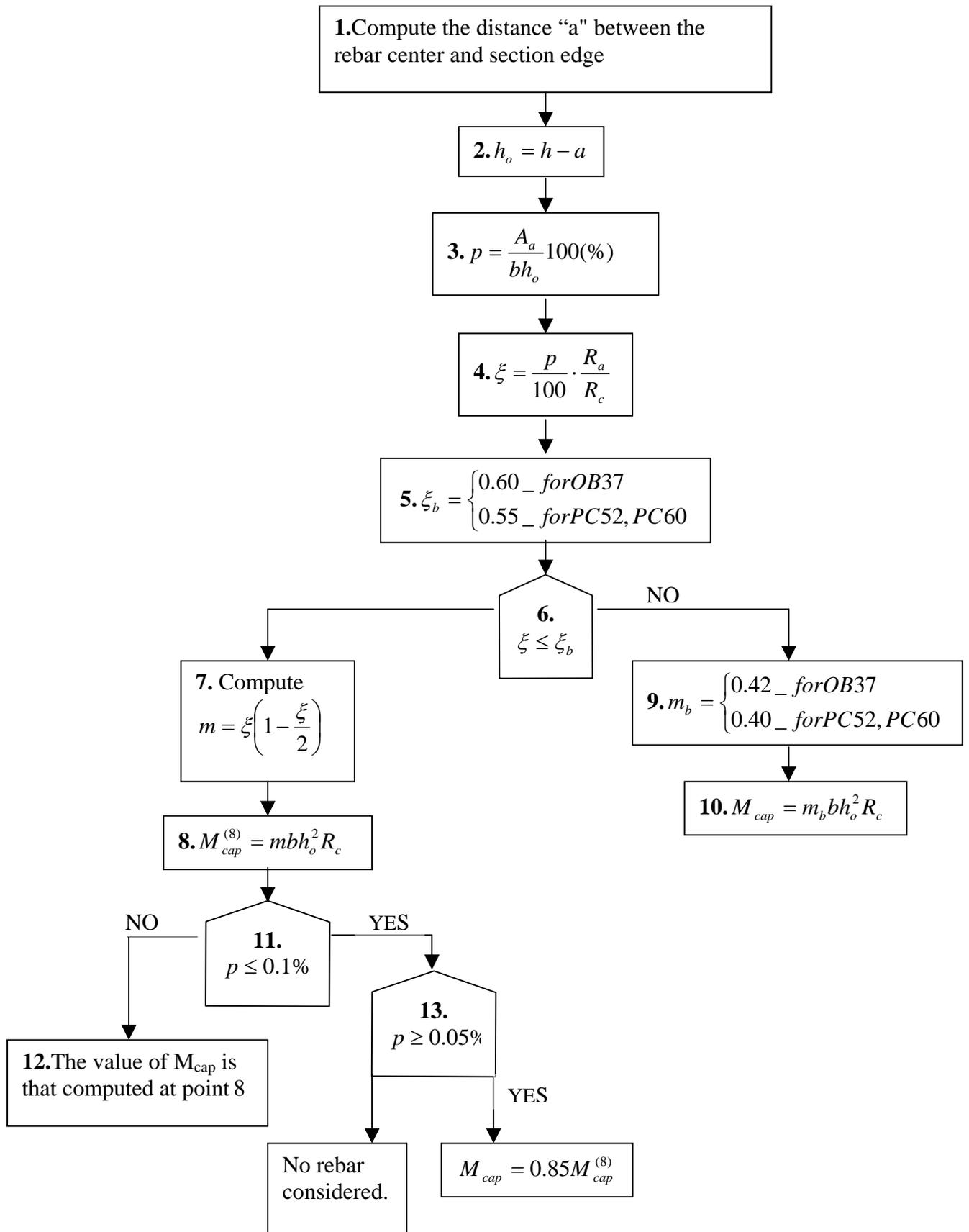
**Figure 24:** Computation of the capable bending moment for a simple reinforced concrete section under pure bending. We know  $b, h, A_a, R_c, R_a$  and we are interested in  $M_{cap}$
