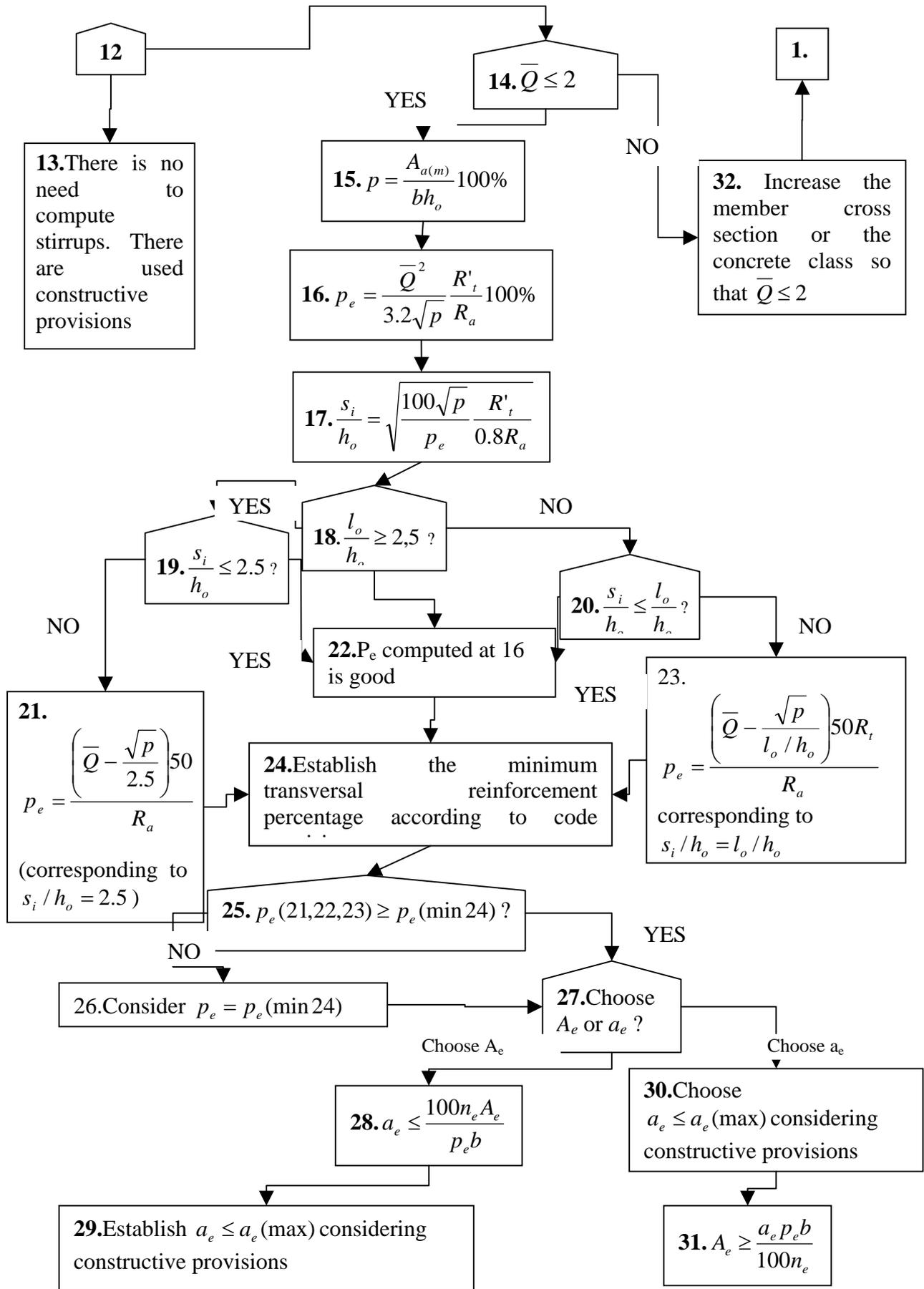
**Figure 27:** Computation of the stirrups for an element with axial force: We know  $b, h, R_t, R_a, N, Q, A_a$  and we are interested in  $A_e, a_e$ .
