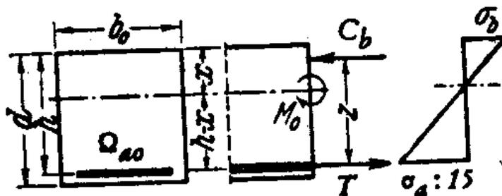
Figure 14: Simple reinforced concrete section
