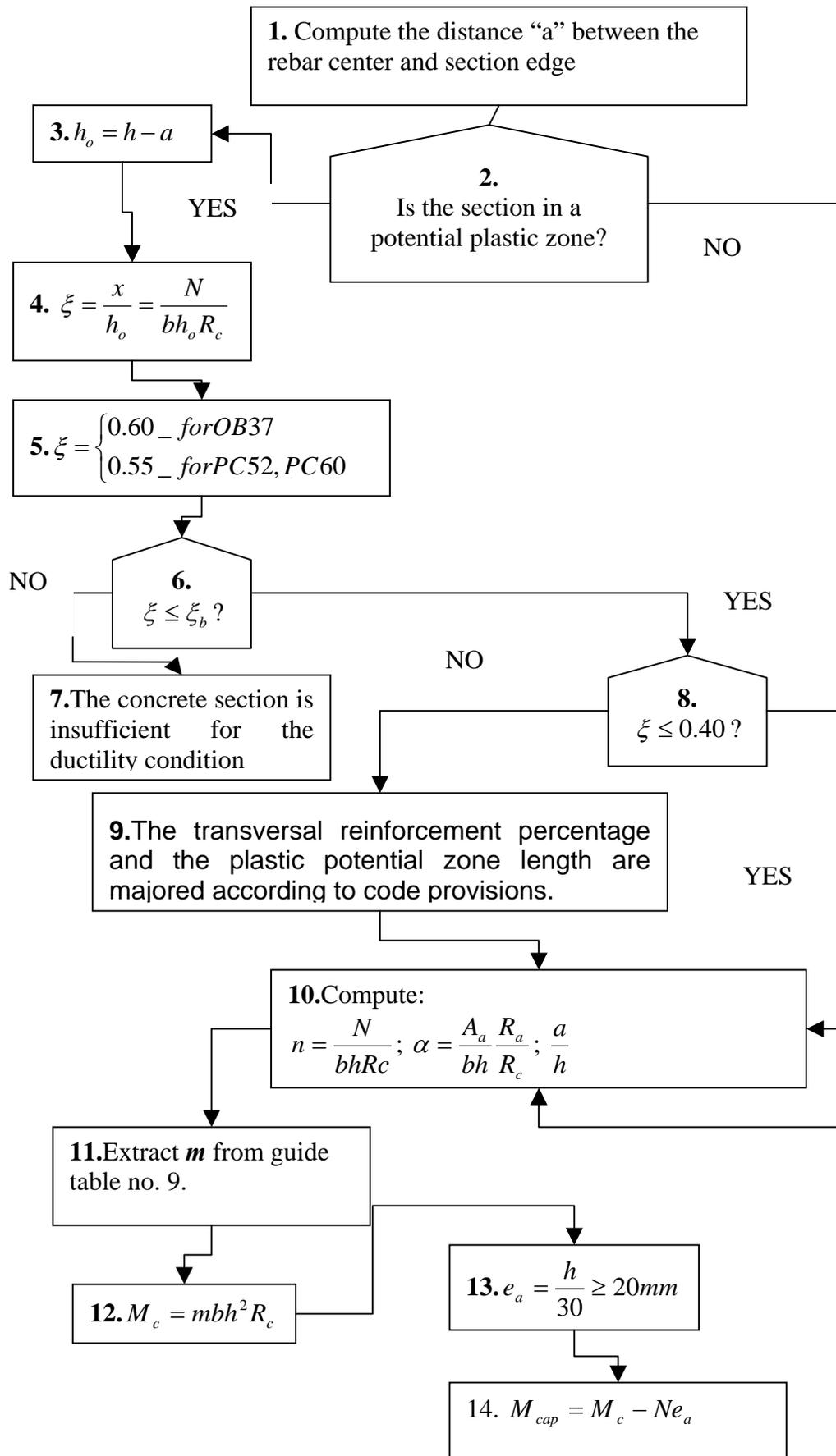
**Figure 25:** Computation of the bending capacity for a column section with eccentricity. We know  $b, h, R_c, R_a, N, A_a = A_a'$  and we are interested in  $M_{cap}$
