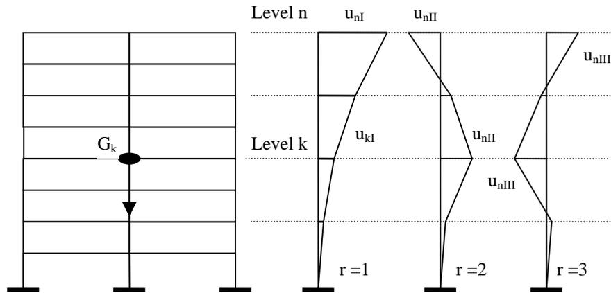
**Figure 5:** First three vibration modes
