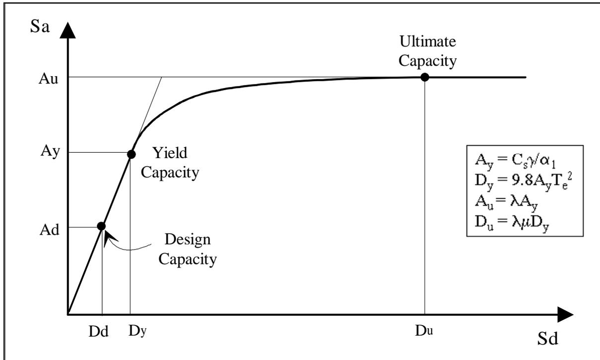
**Figure 8:** Example of Building Capacity Curve
