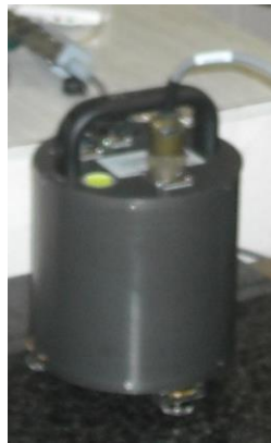
Figure 3. Instruments used at Savo Seismic Station (Guralp Seismometer).
