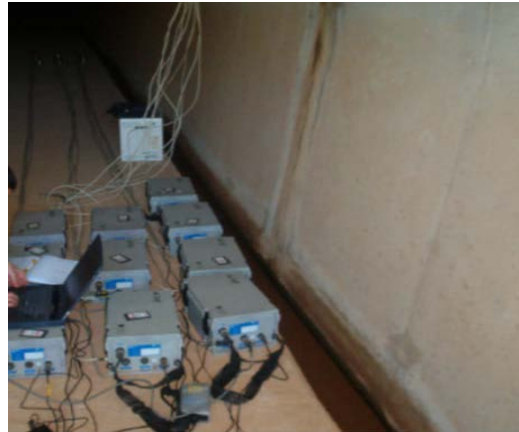
Figure 6. Short Period Stations Data Logger Kinematics K2 Sensor Lennartz LE-3Dlite
