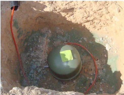
Figure 7. Broad Band Station Sensor Strikisen STS2
