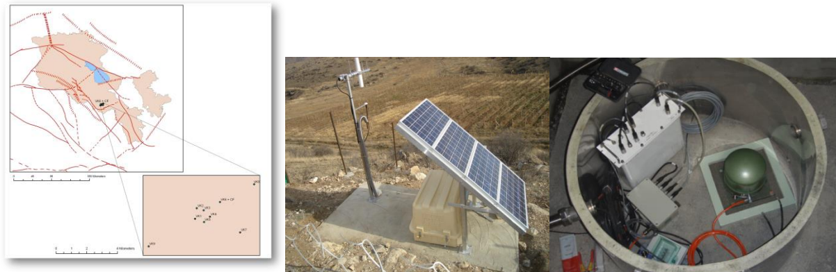
Figure 5. VAYK Seismological Array and STS-2 seismometer
