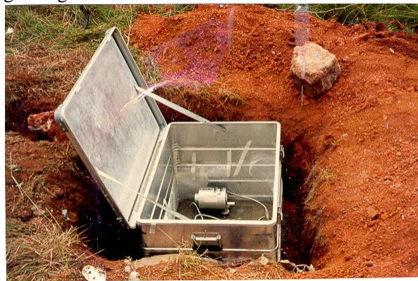
Photo 3. Seismometer installation at Dundu site.
