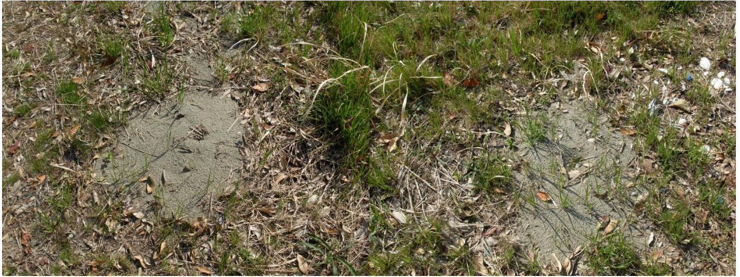
Photo 26. Sand boils was observed. Sand boils are diagnostic evidence of elevated poor water pressure at depth and an indication that liquefaction has occurred.
