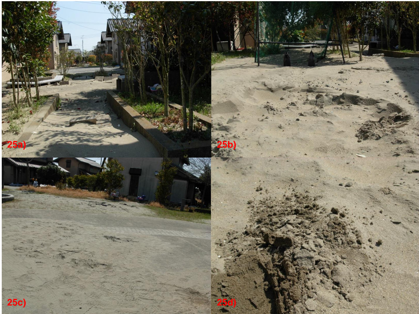
Photo 25a), 25b), 25c) and 25d). Alteration of surface soil characteristics. Before the earthquake this kind of soil (fine sand) there was not on the surface, due to liquefaction phenomenon, the uplift of the underground occurred. The kind of sand is fine sand silty (photo 25d), even on the paving stone the sand came up (photo 25c)
