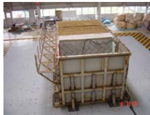
Photo 1 specimen after application of 818 gal
