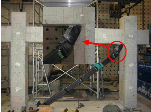
Figure 3 Observed damage of CFT-M18
