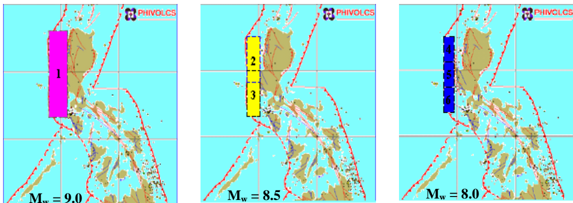
Figure 1 Location of fault plane models for six cases in the Manila Trench area (Sources: Philippine Institute of Volcanology and Seismology , http://www.phivolcs.dost.gov.ph/ ).
