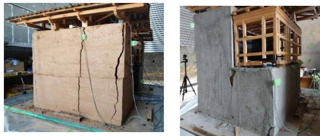
Figure 8. Rammed earth (URE & RRE)
