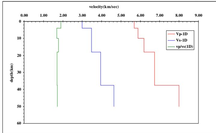
Figure 4. The final 1-D velocity model and the  $V_p/V_s$  ratios for the both models.
