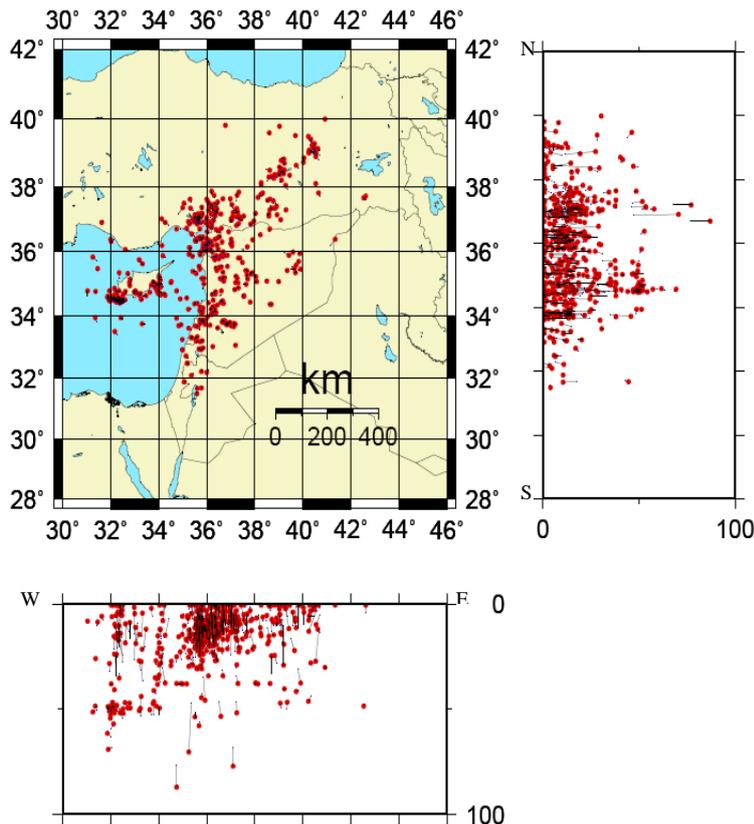
Figure 7. Comparison between the relocated hypocenters by the new velocity model and the hypocenters by the current velocity model.
