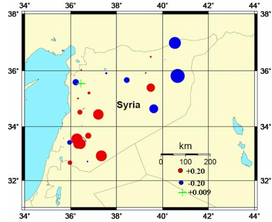
Figure 6. S-wave time station corrections
