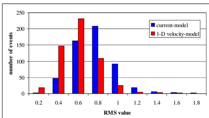
Figure 8. Difference of RMS of the residuals between the hypocenter locations using the current velocity model and the estimated 1-D velocity model
