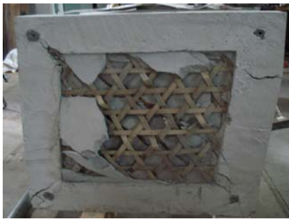
Figure 3 Behavior of Specimen J10BCTP after testing Figure 4 Behavior of Specimen J10BCWP after testing
