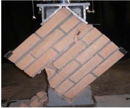
Figure 1 Behavior of Specimen J10B after testing Figure 2 Behavior of Specimen J10B after testing
