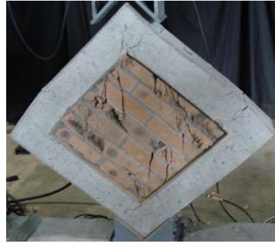
Figure 1 Behavior of Specimen J10B after testing Figure 2 Behavior of Specimen J10B after testing
