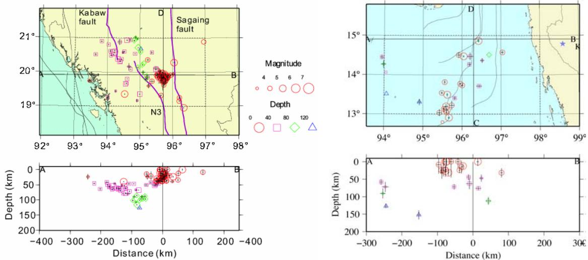
Figure 5. The relocated hypocenters by the MJHD method for region (I). The symbols are the same as in Figure 4b.
