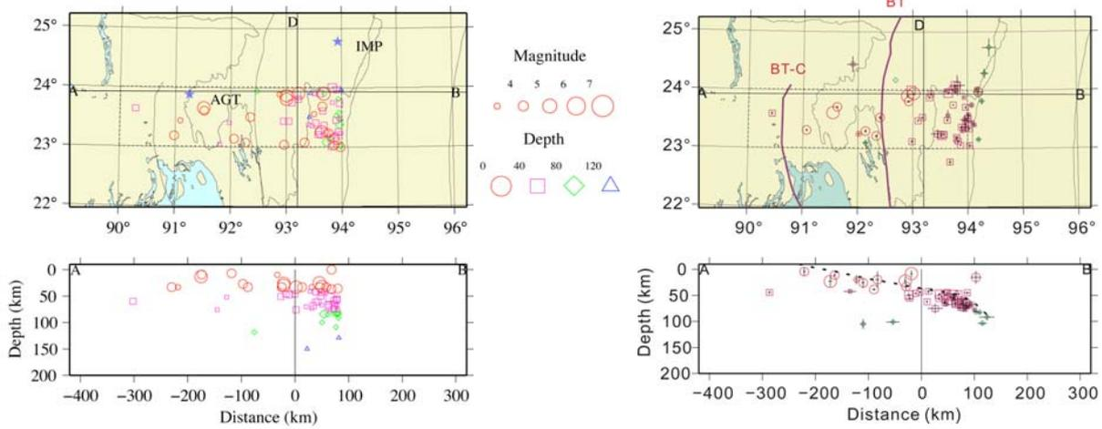
Figure 4a. ISC hypocenter in region (A). The epicenter distribution and two vertical cross sections along A-B and C-D lines are illustrated. A dotted rectangular in epicentral map indicates the epicentral area of selected earthquakes. The size of the symbols represents the magnitude of the events. The color and shape of the symbols denotes the depth range of the events
