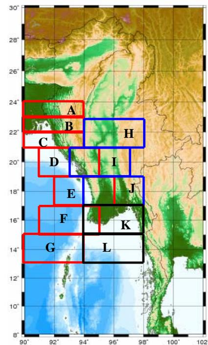
Figure 3. Map showing the 12 sub regions. The rectangulars (A-G) with red color include the Burma subduction zone, the rectangulars (H-J) with blue color include the Burma subduction zone to Sagaing fault and the rectangulars (K-L) with black color include the Southern opening zone.
