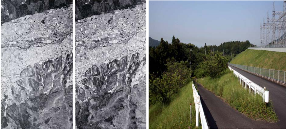
Figure 1 Left) Aerial photographs of the Hatano fault, Doi area, MTL. Right) The Road constructed on the scarp of the Hatano fault which shows prominent offset of ridge and valley. Topography is artificially changed and a substation was constructed.
