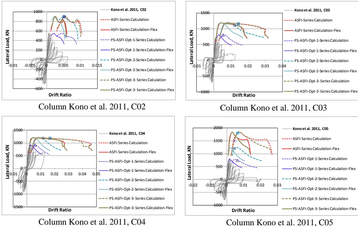
Figure 3. Backbone curve and ultimate point for selected columns using ASFI and three different options of concrete compression softening.
