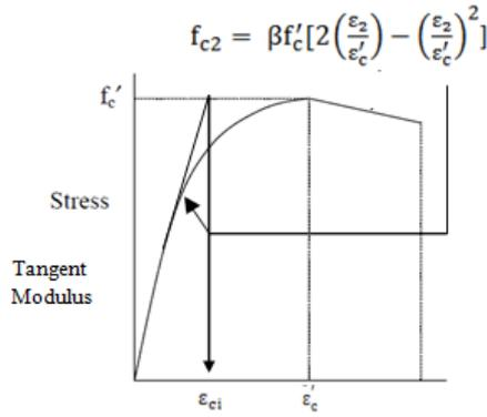
Figure 2. Determination of strain level for developing different options for parametric study in the stress strain curve of concrete
