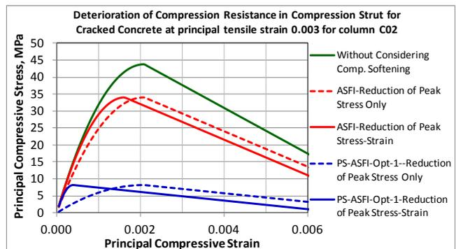
Figure 4. Deterioration of compression resistance in compression strut for cracked concrete at an arbitrary point of large principal tensile strain for column C02
