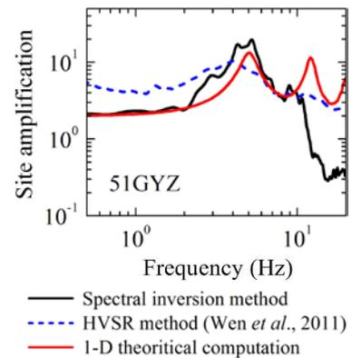
Figure 2. Site response of the station 51GYZ calculated by three methods
