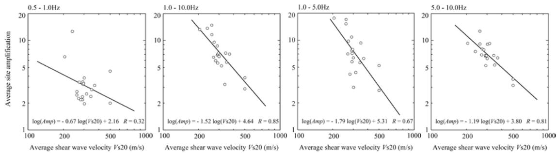
Figure 5. Average site amplification for 0.5-10.Hz, 1.0-10.0Hz, 1.0-5.0Hz and 5.0-10.0Hz frequency bands as a function of  $V_s20$
