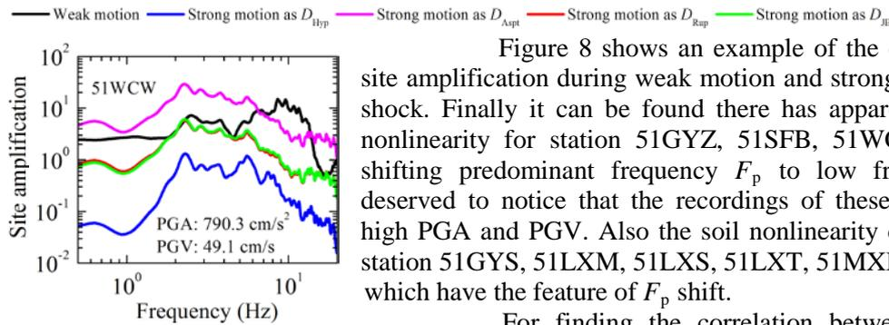
Figure 8. The example of the comparison between site amplification during weak motion and strong motion in the main shock of Wenchuan Earthquake
