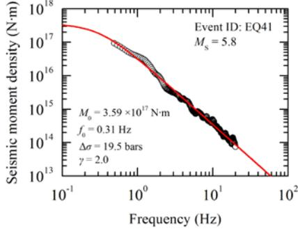
Figure 10. The inversed (circles) and the best-fitting (red line) seismic moment density for an exemplified event
