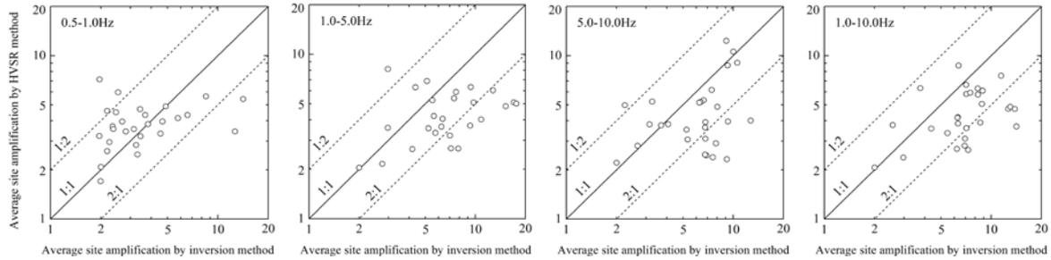
Figure 4. Comparison of the average site amplification calculated by spectral inversion method and HVSR method for each frequency band
