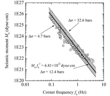
Figure 11. Seismic moment versus corner frequency obtained from inversion analysis. The shaded area of this figure means the area of one standard deviation of the mean value. Eq. (5) also can be written as  $M_0 f_0^3 = 6.76 \times 10^{22}$  dyne·cm corresponding to a constant stress drop 12.4 bars.
