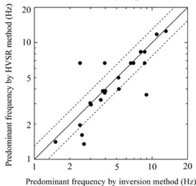
Figure 3. Comparison of the predominant frequency calculated by spectral inversion method and HVSR method
