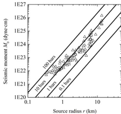
Figure 12. Seismic moment versus source radius for each event
