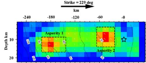
Figure 7. Two asperities were identified for Wenchuan Earthquake. Fault slip model is derived from USGS.
