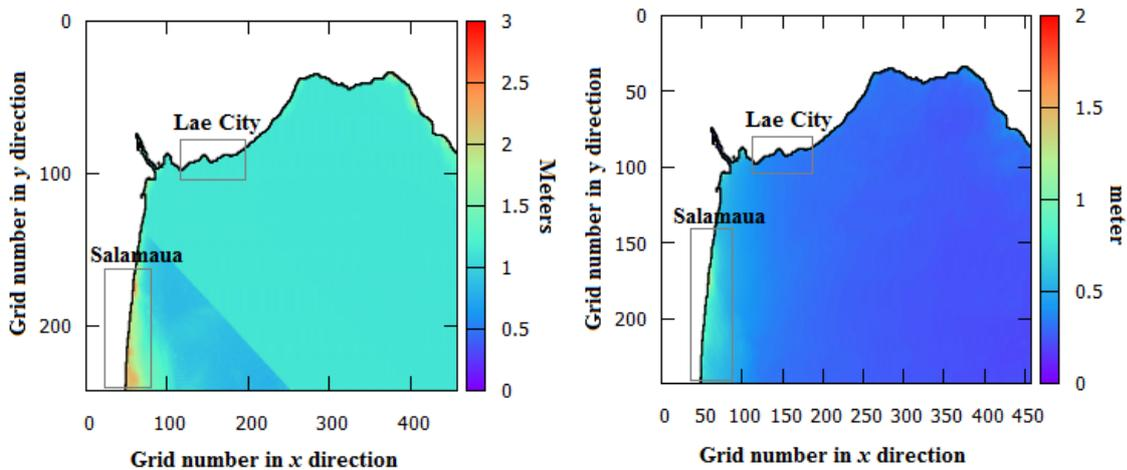
Figure 6. Calculated tsunami inundation of the region 4 from earthquake scenarios Mw8.6 S1 (left) and Mw8.1 SA (right).
