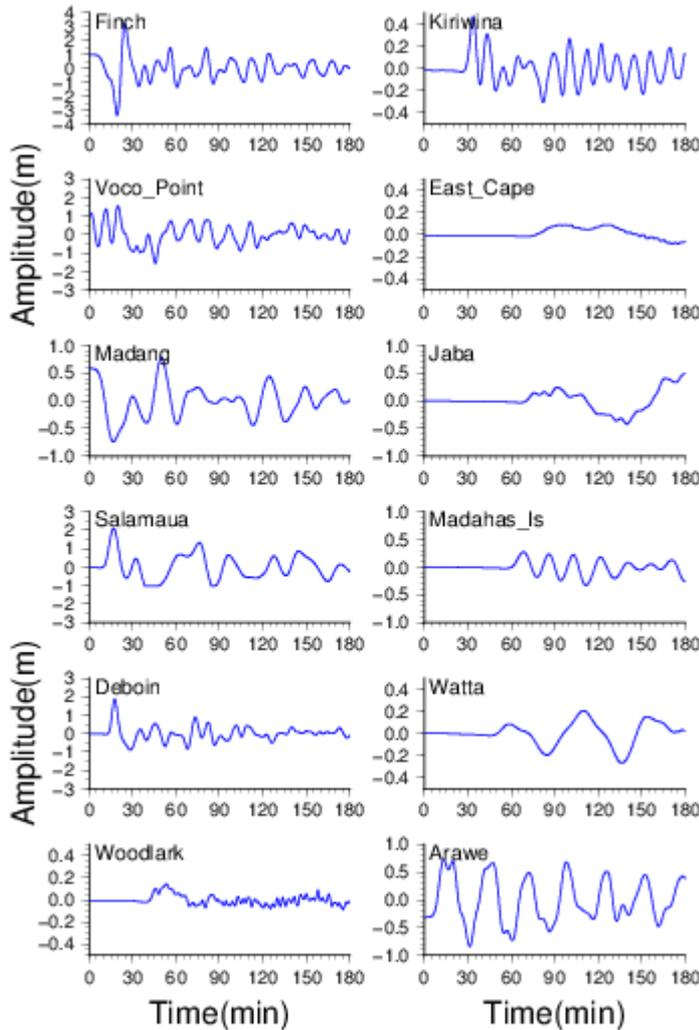
Figure 3. Calculated tsunami waveforms for each coastal point for the earthquake scenario Mw8.6 S1.
