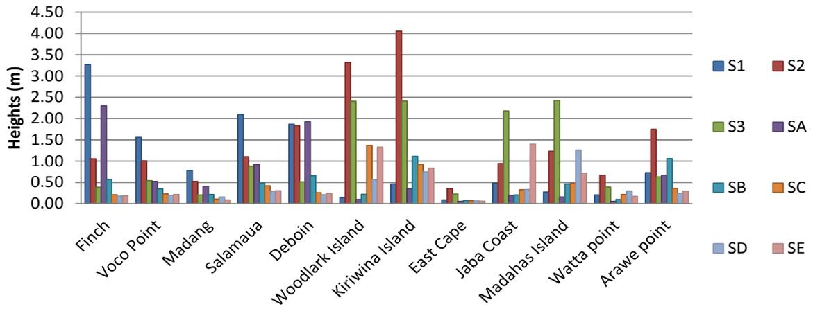
Figure 4. Tsunami heights for each coastal point from the computation of the earthquake scenarios.
