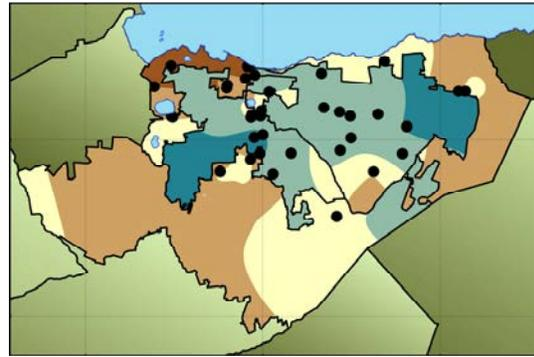
Figure 2. Soil classification map based on Vs-20 analysis of Managua.
