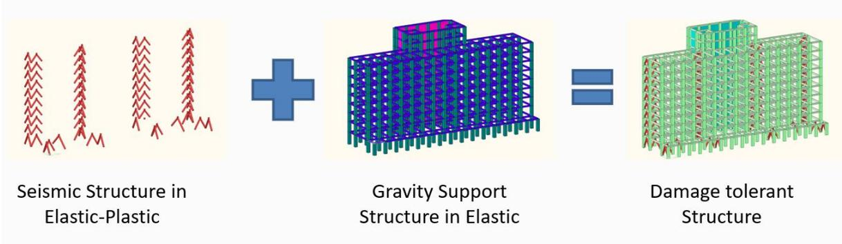
Figure 3. Retrofit Strategy using steel damper, ADAS.
