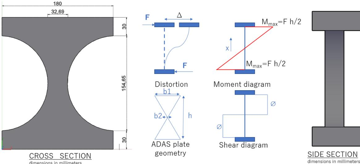
Figure 1. Moment and bending deformation of ADAS Steel Damper due to lateral force.
