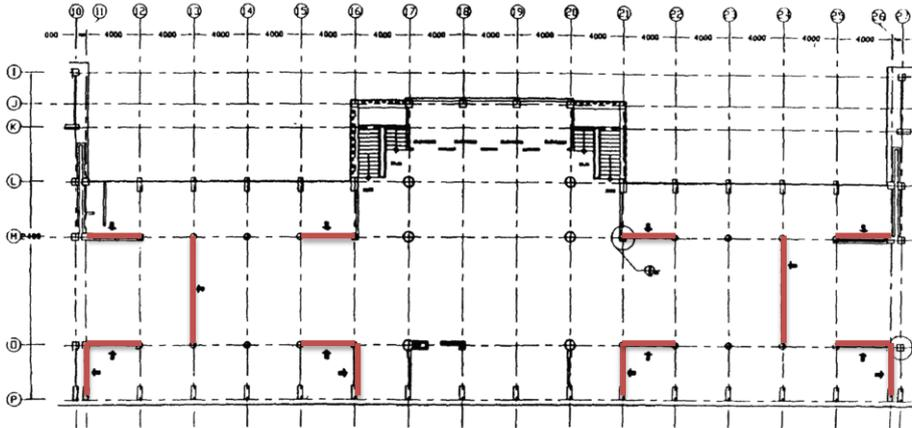
Figure 2. Plan of target building and arrangement of ADAS steel dampers.
