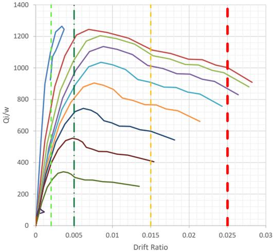
Figure 5. Shear force - story drift angle (Before retrofit).
