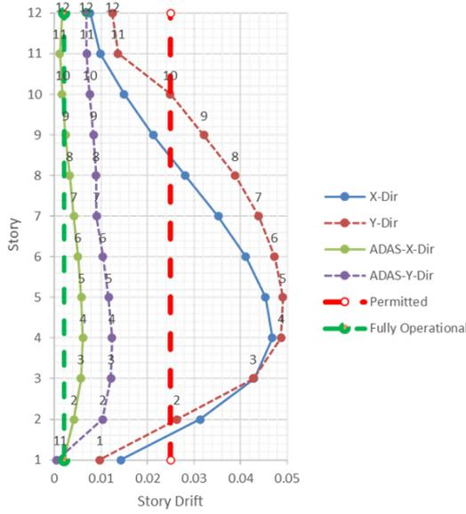
Figure 7. The maximum story drift of target model before and after retrofit.
