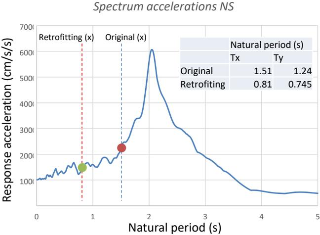
Figure 4. Response acceleration spectrum, and natural periods of target model before and after retrofit.
