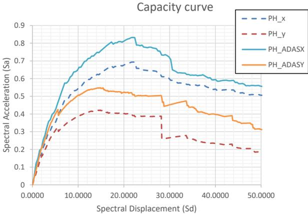
Figure 6. Capacity curves of target model before and after retrofit.
