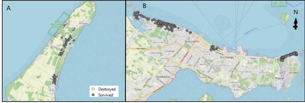
Figure 2. Spatial distribution of damaged buildings in (A) Hihifo and (B) Nuku'alofa areas. It shows the destroyed buildings (white dots) and survived buildings (grey dots).
