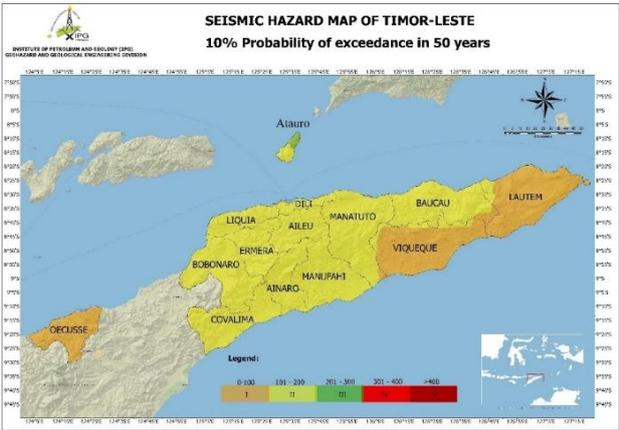
Figure 1. Peak ground acceleration for 2% and 10% probability of exceedance in 50 years.
