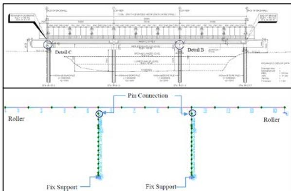
Fig. 1. Analyses Model of the target model bridge.
