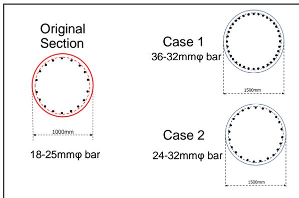
Fig. 2. Details of the Original Sections and the Revised Sections
