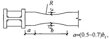
$$b = (0.65 \sim 0.85)h_b, \quad c = 0.25b_f, \quad R = (4c^2 + b^2)/8c, \text{ 切割面应刨光}$$
