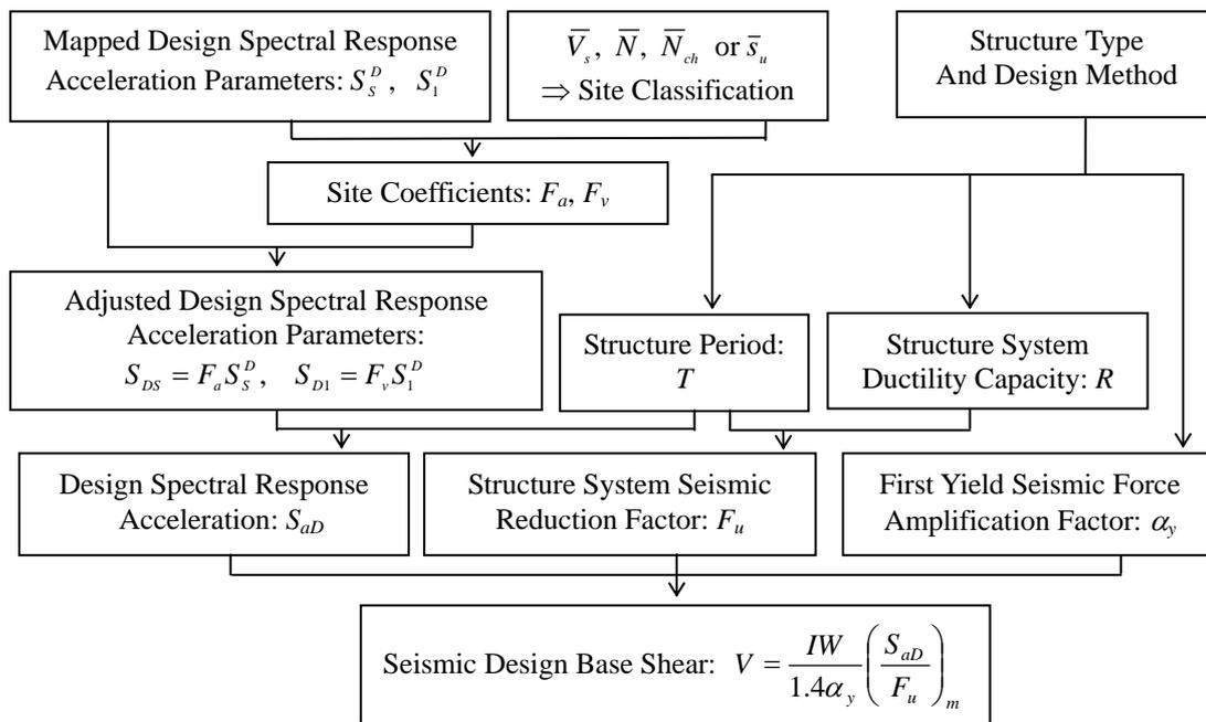
Figure 2. Procedures to determine the seismic design base shear for general sites
