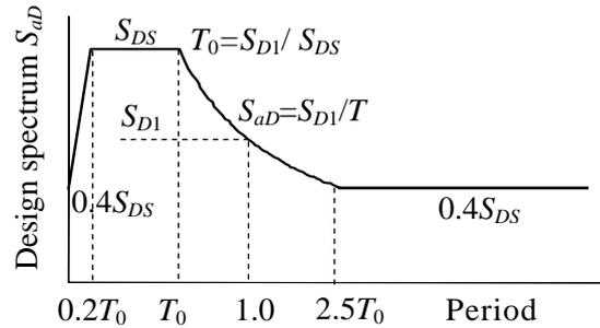
Figure 1. Design response spectrum developed from the site-adjusted parameters  $S_{DS}$  and  $S_{D1}$
